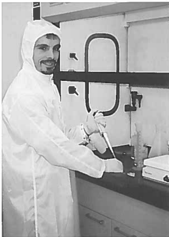
Tom Johnson working in his “clean lab.” Because the samples he works with are so infinitesimal, the slightest dust particles can contaminate his work. Johnson wears special clothes, including shoes, to work in this lab.
