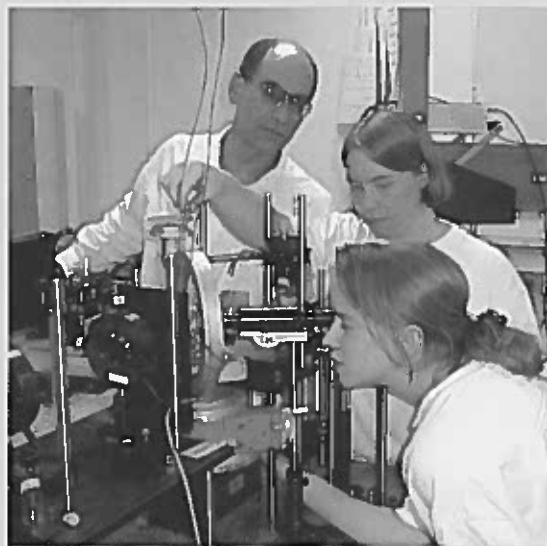
Jay Bass, Megan Elwood and Jennie Jackson examine work at the Brillouin Laser Light Scattering apparatus which measures sound wave velocities in minerals.
