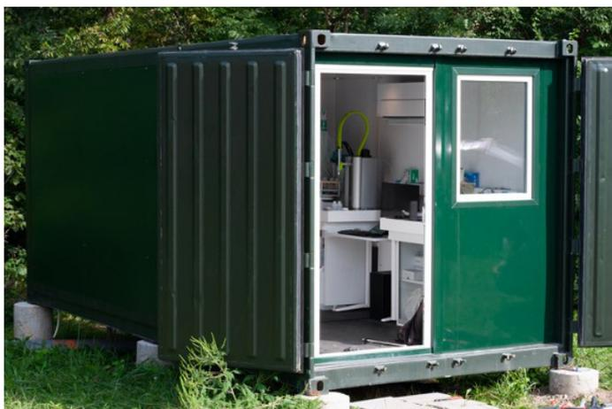
*The River Lab, located in Monticello, Illinois, performs automated chemical analyses of Sangamon River water several times per hour to catch all the nuances of water and solute dynamics in the watershed.*
